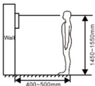
The camera should be 1450~1550mm above the ground.
