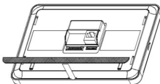
Align the edge of the silica gel pad with the lower edge of the casing, and paste the pad.
