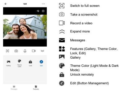
enter the interface of monitor. Resident can make a video call to Door Station and unlock remotely on the smartphone. If Door Station is calling in, Indoor Monitor and Smart Life App can ring at the same time, and the mobile phone APP can answer the call and unlock remotely. Smart Life App can also monitor and unlock Door Station.
