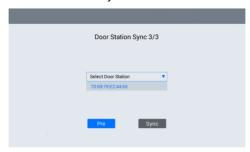
Step 5: Network of subordinate Indoor Monitor can be either dynamic or static. Select DHCP to enable dynamic network or fill in IP, Mask and Gateway to set up static network for subordinate Indoor Monitor. Network segment should be the same as first Indoor Monitor's when using static IP address. For example, IP address should be 192.168.0.\*\*if IP address of first Indoor Monitor is 192.168.0.\*\*.
