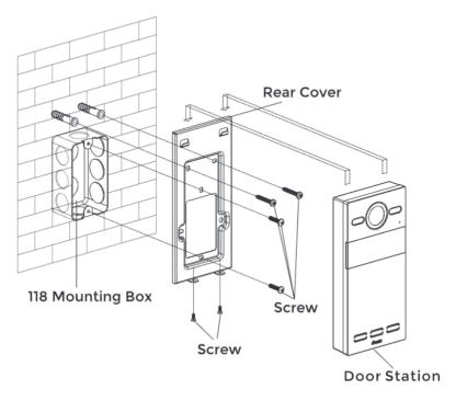
Product size:  $88 \times 168 \times 32.5$  mm Surface Mounting size:  $88 \times 168 \times 34$  mm
